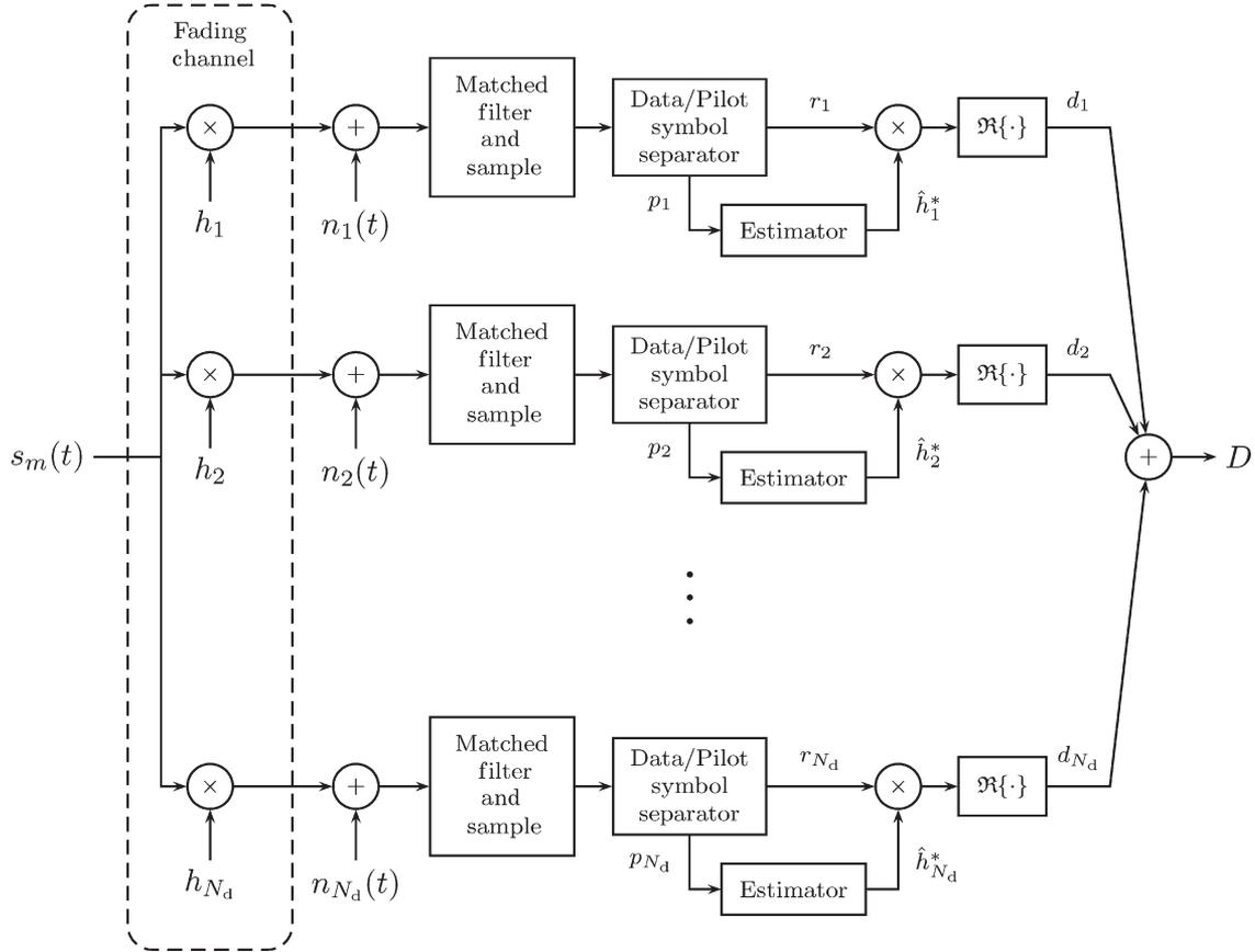
Fig. 1. Diversity system utilizing practical channel estimation.
