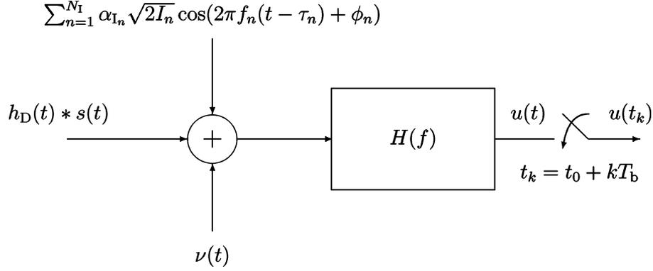
Fig. 1. System with multiple tone interferers and additive noise.
