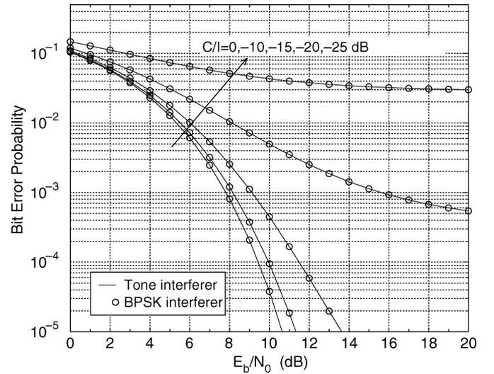
Fig. 4. BEP for the TH-PPM system considered in the unfaded/faded scenario with a single tone interferer. Analytical results are also compared with the simulation for a 1 Mb/s BPSK interferer.
