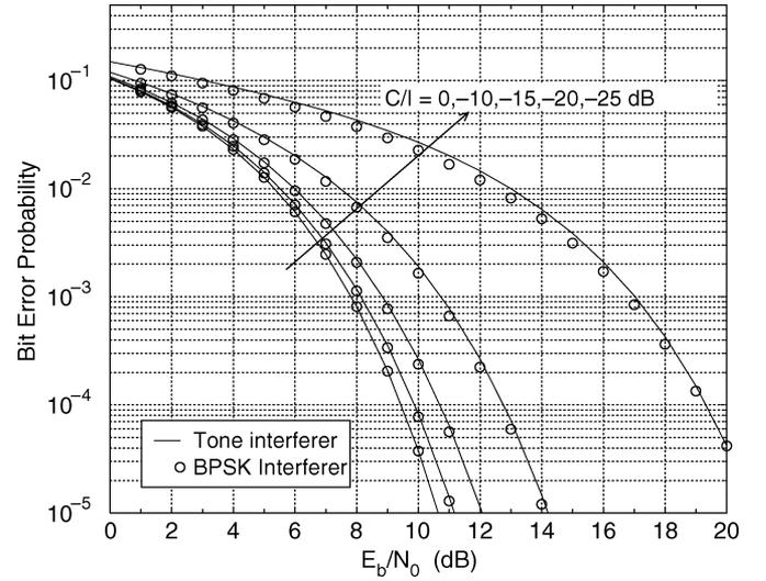
Fig. 3. BEP for the TH-PPM system considered in the unfaded/unfaded scenario with a single tone interferer. Analytical results are also compared with the simulation for a 1 Mb/s BPSK interferer.
