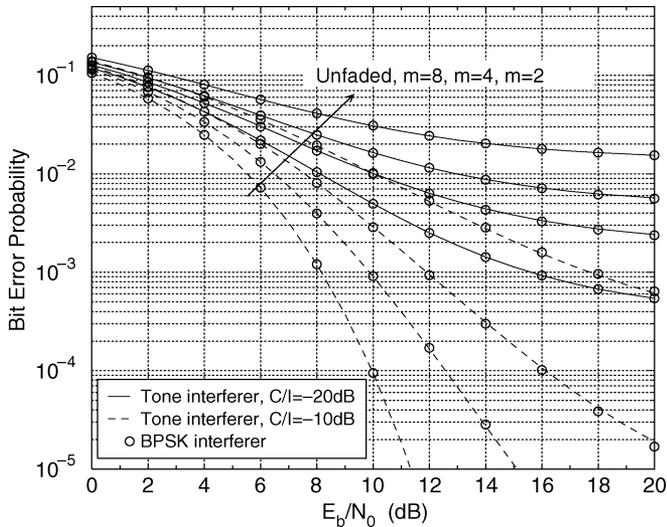
Fig. 5. BEP for the TH-PPM system with a single tone interferer in the faded/faded scenario, for different values of  $m$  and for the unfaded/faded case, i.e.,  $m = \infty$ . Analytical results are compared with simulations for a 1 Mb/s BPSK interferer.
