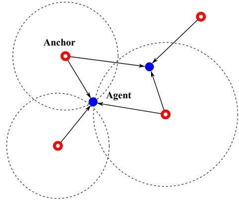
Fig. 1. Network deployment for WNL: agents (blue dots) determine their positions based on range measurements with respect to anchors (red circles).
